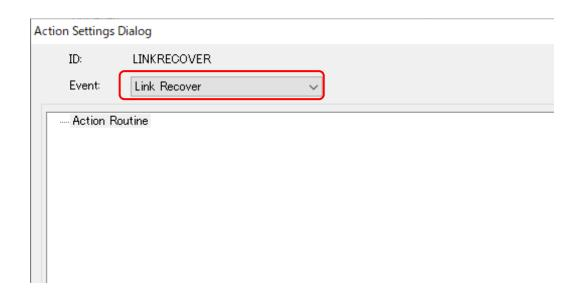
For example, with this setting, it is possible to clear the error screen when the communication error is recovered.
