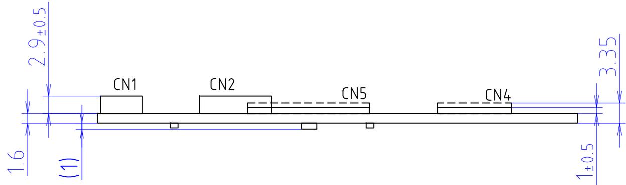
TOLERANCE =  $\pm 0.3\text{mm}$  except for hole diameter
