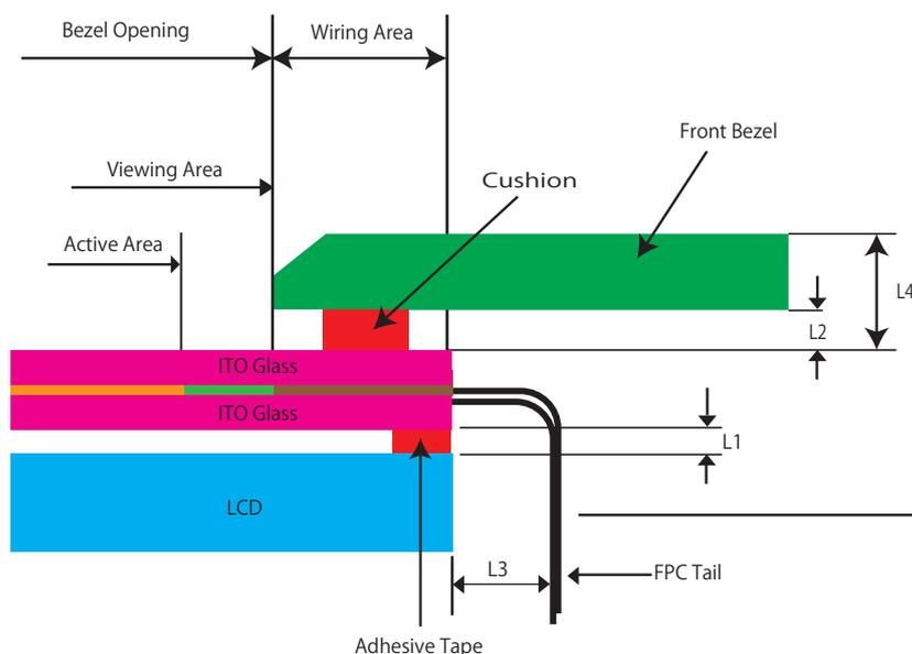
$L4 \geq 2\text{mm}$ : Distance between touch screen and bezel surface
