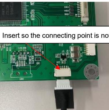
Insert so the connecting point is not visible.
