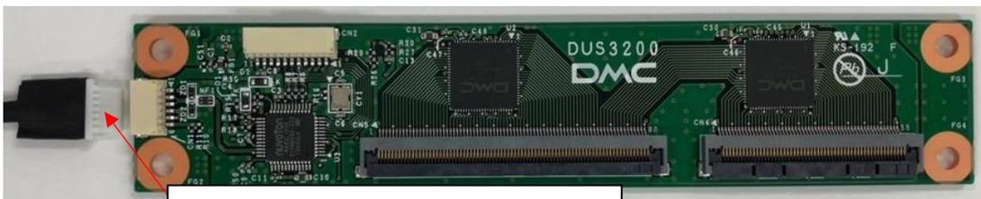
Insert so the connecting point is not visible.
