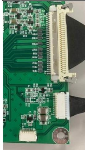
Insert with the connecting point facing up not visible.
